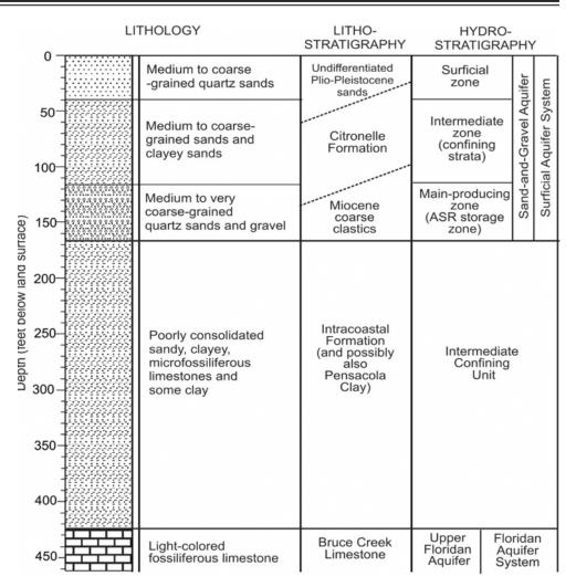
Figure 2. Hydrostratigraphic column for the aquifer storage and recovery system vicinity.
