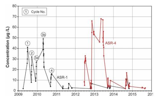
Figure 4. Arsenic concentrations of recovered water from wells ASR-1 and ASR-4.
