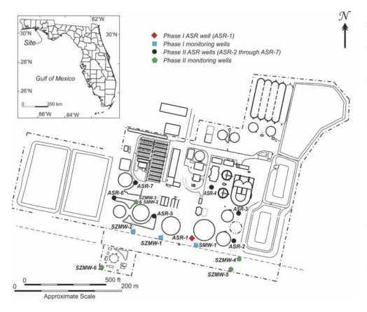
Figure 1. Site location map and site plan showing the locations of the aquifer storage and recovery wells, storage zone monitoring wells, and shallow monitoring wells.
