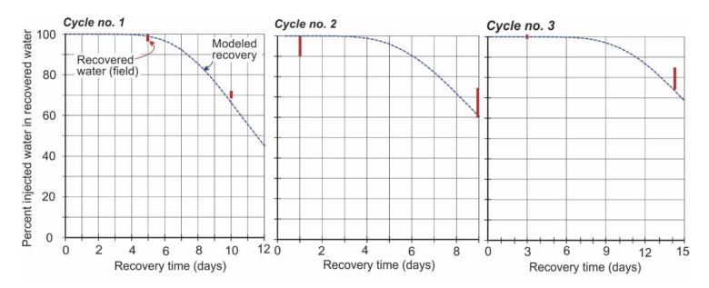
Figure 3. Modeled versus actual recovery of recharged reclaimed water.
