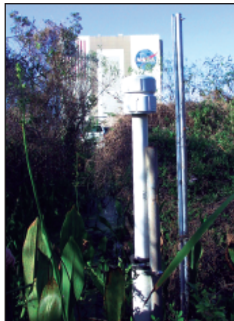
One of four water level recorders at the VAB Wetland Site.
