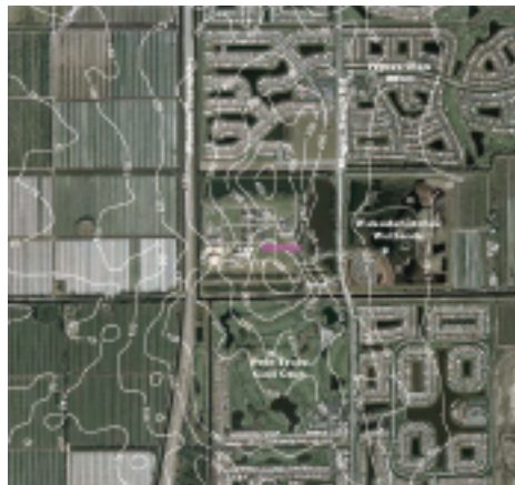
Figure 3 Baseline Peak D/T Contours Aeration Basin Sources
