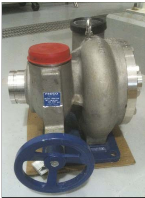
Figure 3. Reverse Osmosis Energy Recovery Device
