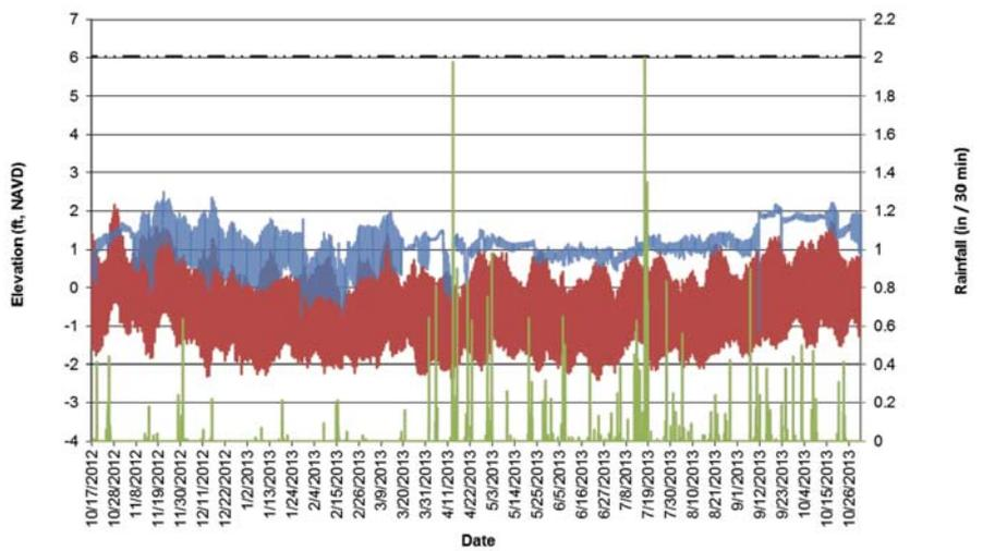
Figure 12. From November 2012 to March 2013, the convention center site groundwater levels varied at about 0.5 times the tidal amount, the most for any site. However, the high groundwater levels fluctuated with tides, but were about 1 ft above the tidal elevations.
