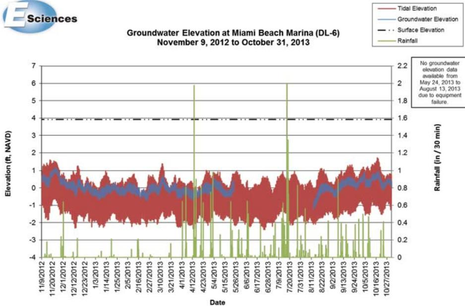
Figure 10. The Miami Beach Marina site shows that the groundwater level fluctuated 0.3 ft with the tidal cycle, with the peaks at or within 0.5 ft of high tide.
