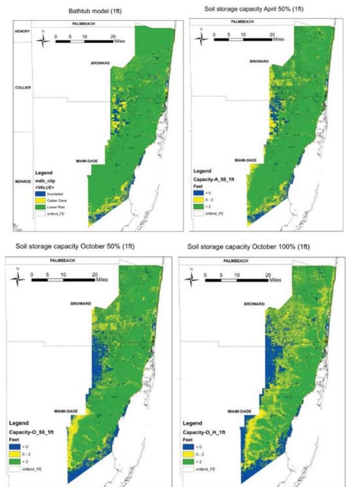
Figure 2a. This shows the bathtub results model (current condition), while 2b-d show soil storage capacity with 1-ft sea-level rise.
