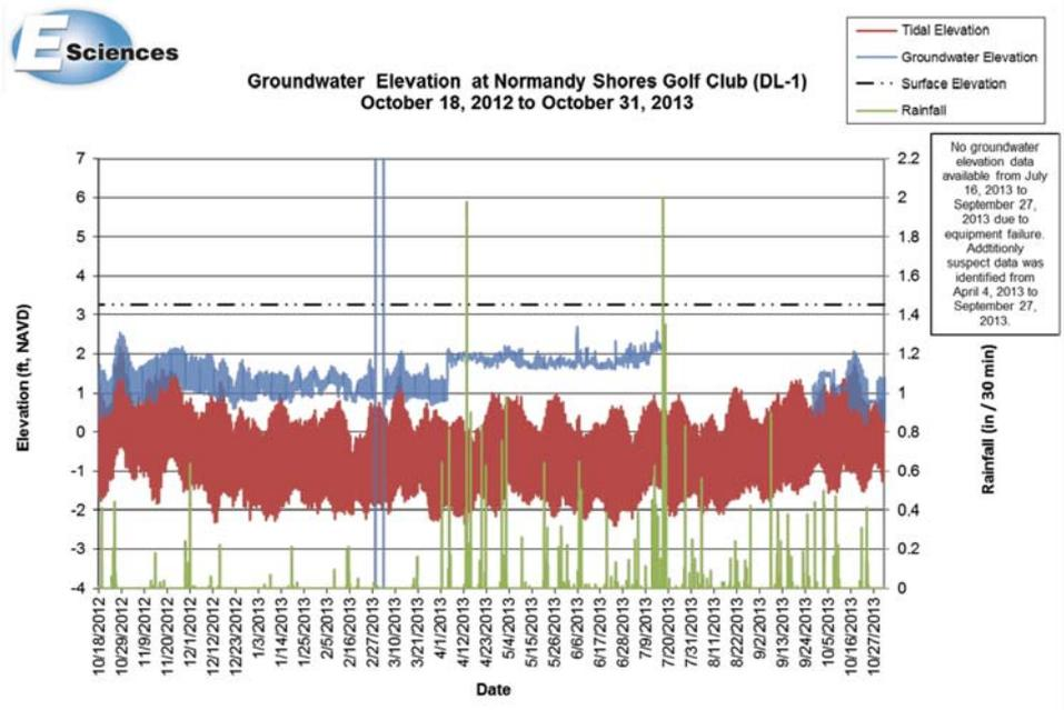
Figure 9. The Normandy Shores Golf Course site is artificially irrigated. This site shows that for the first six months of monitoring, the groundwater level fluctuated between 0.5 and 1 ft with tides, but while irrigating, remained 0.5 ft above high tide. In October, the end of the rainy season, the tides and groundwater levels correspond.
