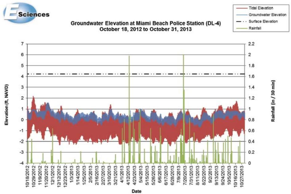
Figure 8. The Miami Beach Police Station site shows that the groundwater level basically matched the high tide, but fluctuated 0.5 ft downward as tides went out.
