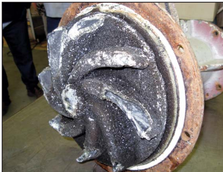
Figure 1. Struvite accumulation on the impeller of a post-digestion biosolids decant pump.
