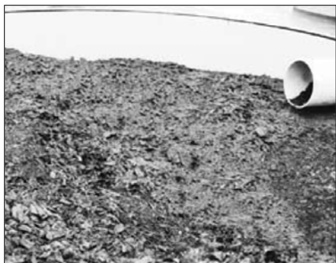
Figure 4. Iron sponge (wood chips impregnated with rust).
