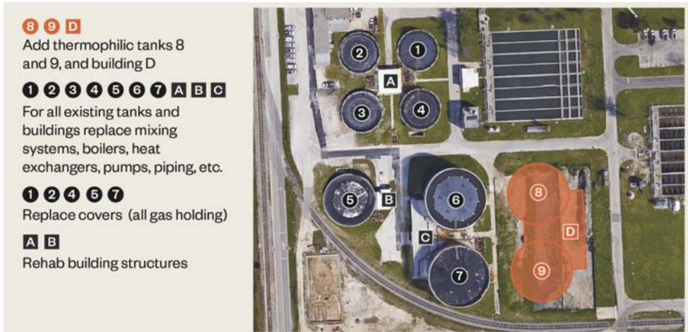
Figure 3. Site Plan: Proposed Temperature-Phased Anaerobic Digestion Facilities
