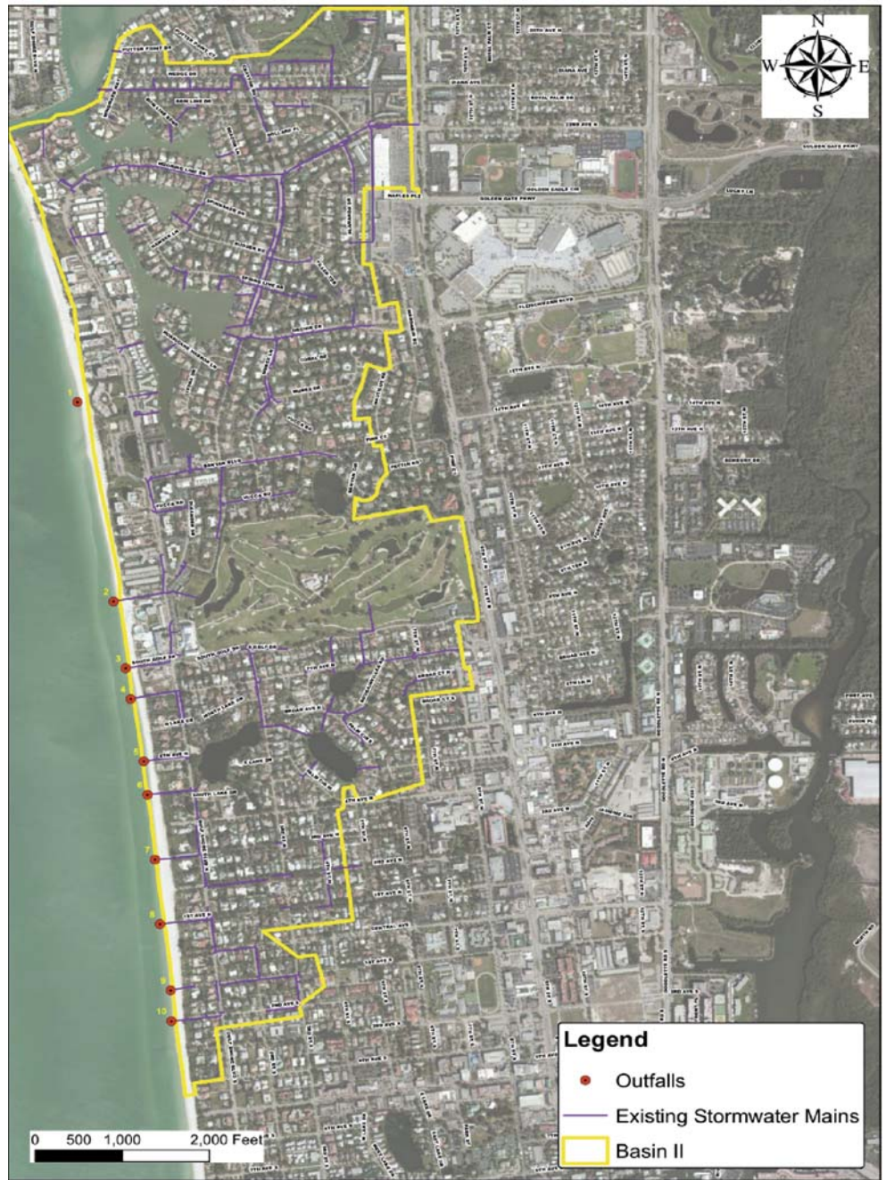
Figure 1. Existing Beach Outfall Locations
