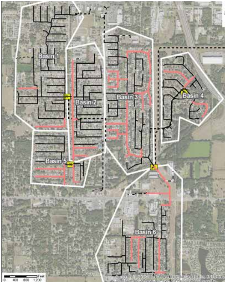
Figure 5. Clair-Mel Collection Network indicating the portion of the network where focused electrode leak location inspection was performed.
