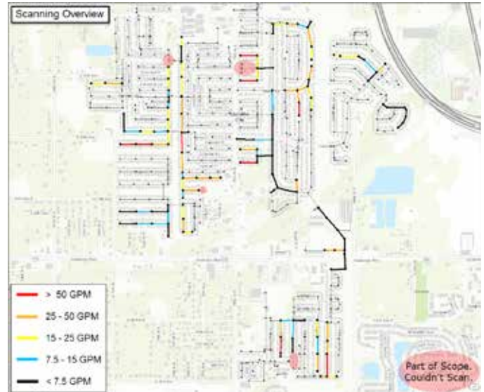
Figure 6. Clair-Mel electrode leak location inspection results showing individual pipes with greatest potential defect flow rates contributing to inflow and infiltration.
