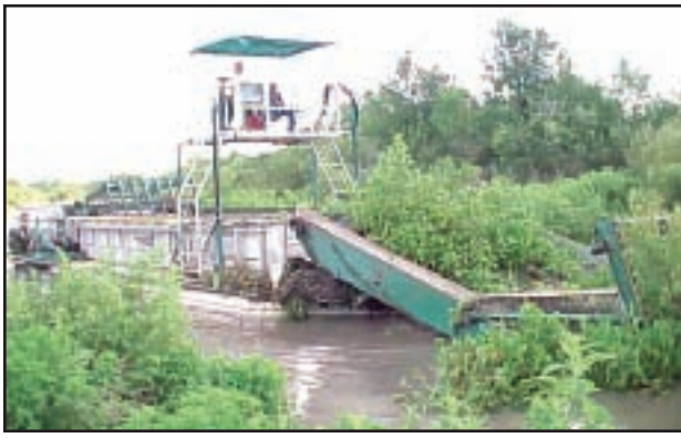
Figure 3 – Mechanical Harvester Removing Aquatic Plants (Texas Aquatic Harvesting Inc. 2007)
