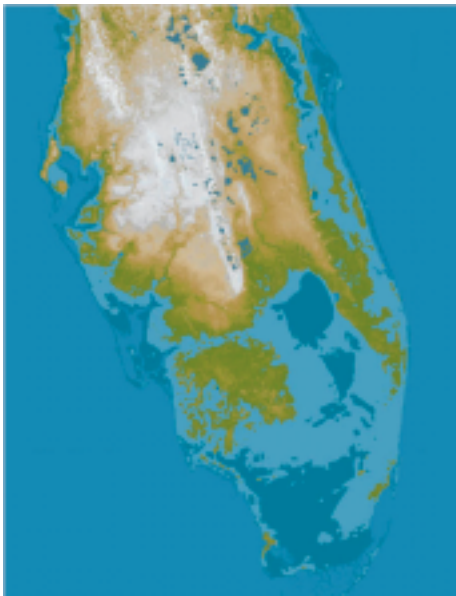
Figure 4 – Sea-level rise impacts (dark blue areas show a sea-level rise of zero to five feet, the most likely scenario, with the higher-risk alternative of five to 16 feet shown in light blue) http://www.nasa.gov/centers/jpl/news/gracef-20060602_prt.htm .
