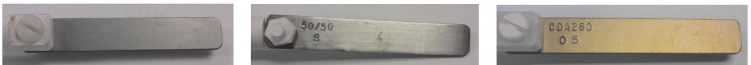
Figure 3. (a) Mild Steel, (b) Lead Solder, and (c) Copper Coupons
