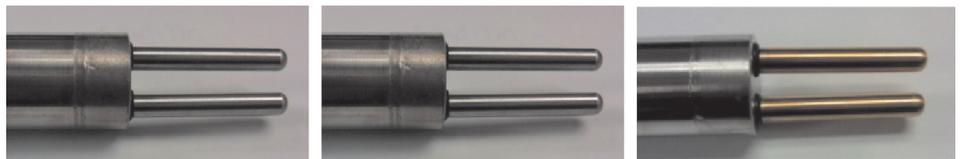
Figure 2. (a) Mild Steel, (b) Lead Solder, and (c) Copper Electrodes
