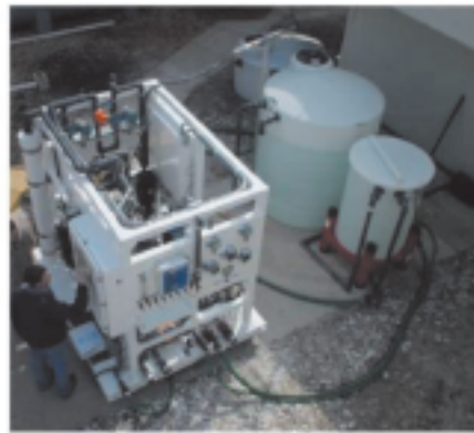
Figure 1: Ultrafiltration pilot during factory testing at Harn R/O Systems Inc. (left) and installed at the Lake Manatee Water Treatment Plant in Manatee County (right)
