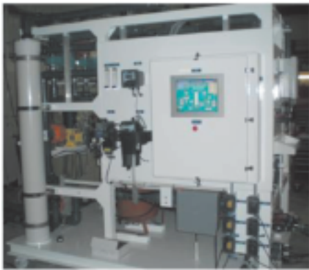
Figure 1: Ultrafiltration pilot during factory testing at Harn R/O Systems Inc. (left) and installed at the Lake Manatee Water Treatment Plant in Manatee County (right)
