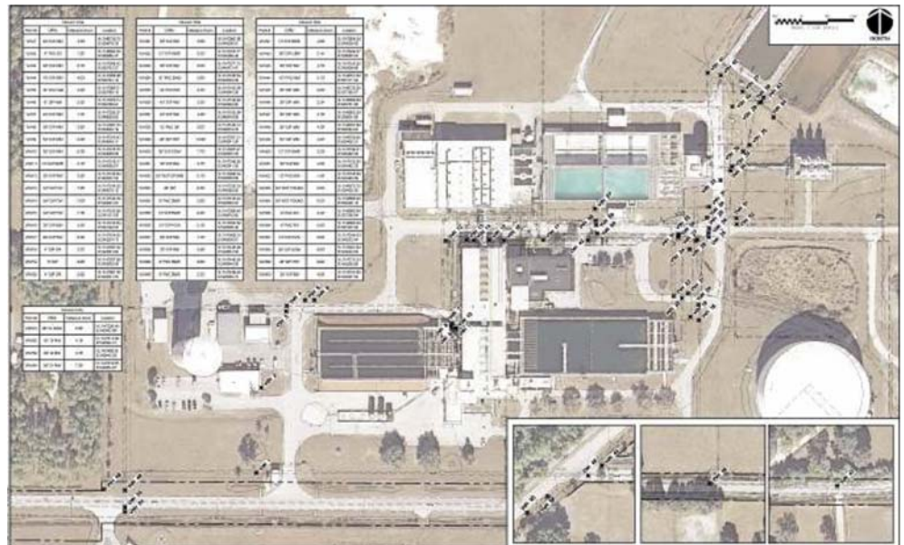
Figure 4. Subsurface Utility Engineering Locates
