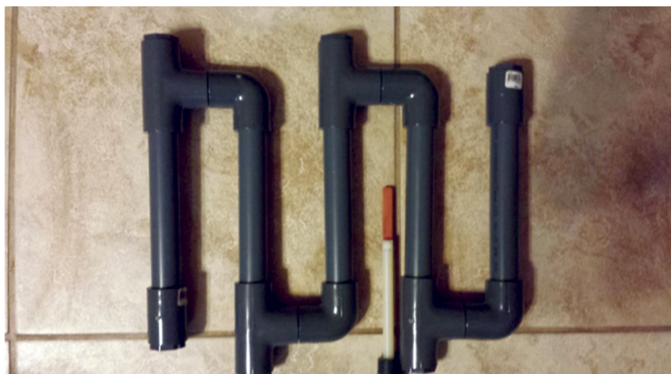
Figure 3. Metal Coupon Test Rack Component Use of coupons provides an average weight loss value. Coupons can also be analyzed for surface characteristics [“cook and look”]. (photo: Benjamin A. Yoakum)
