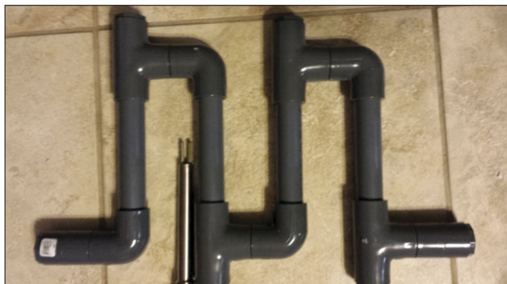
Figure 4. Linear Polarization Probe Test Rack Component The change in resistance of the electrochemical probe over time is measured; the rate of change is directly proportional to the corrosion rate in mils per year. (photo: Benjamin A. Yoakum)
