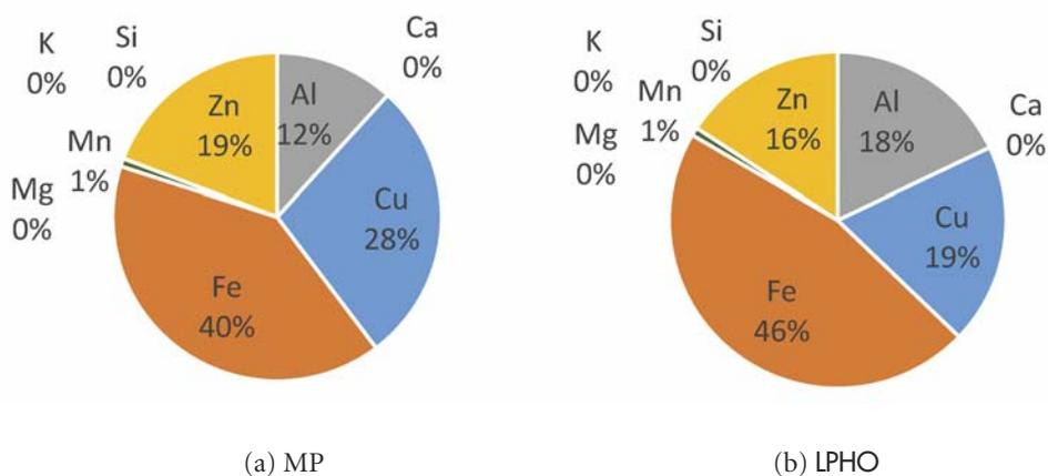
Figure 10. Foulant Characterization on the Sleeve Acid Rinsate – End of Phase 2
