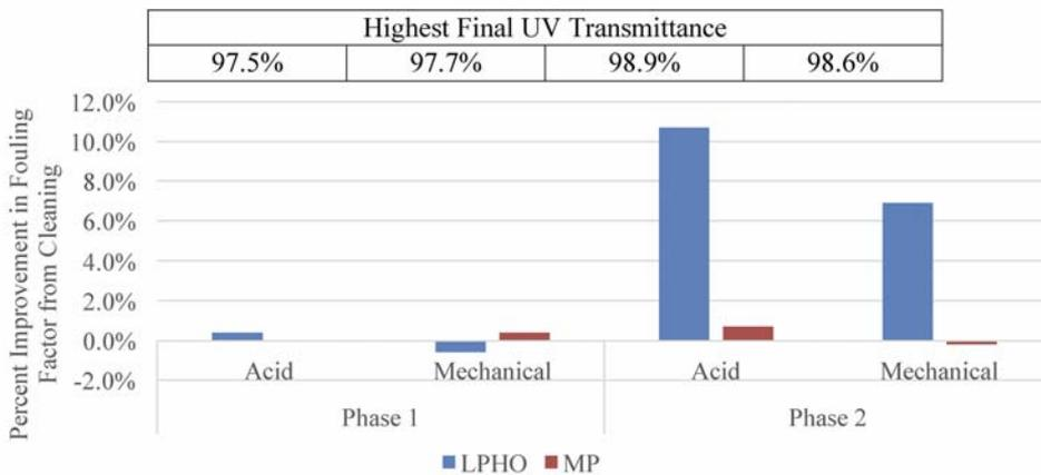
Figure 12. Comparison of Ultraviolet Sleeve Cleaning Methods
