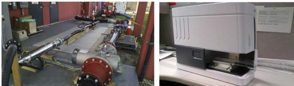
(a) Ultraviolet Pilot Setup and (b) Cary 60 Optics Bench for Measurement of the Ultraviolet Sleeve
