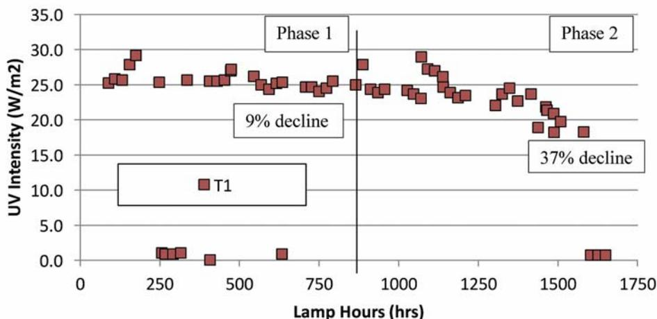
Figure 4. Ultraviolet Intensity Sensor Measurements for Low-Pressure High-Output Reactor
