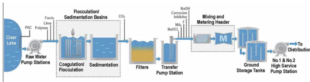
Figure 1. Simplified Existing Treatment Plant Process Flow Diagram
