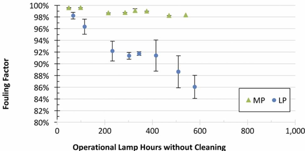
Figure 7. Ultraviolet Reactor Sleeve Fouling for Phase 2 – No Cleaning
