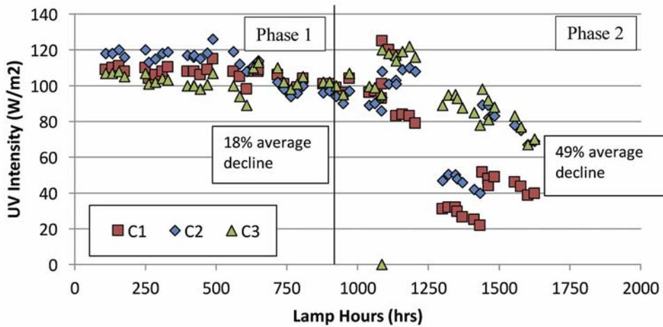
Figure 5. Ultraviolet Intensity Sensor Measurements for Medium-Pressure Reactor
