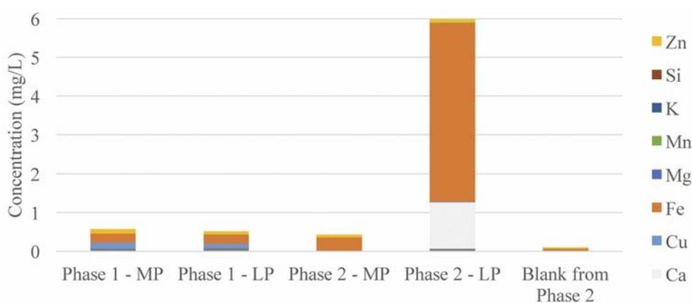
Figure 8. Concentrations of Metals in the Acid Rinsate
