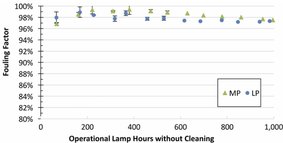
Figure 6. Ultraviolet Reactor Sleeve Fouling for Phase 1 – No Cleaning
